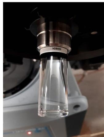
Figure 3: Photo of the vial after completion of 115 days of testing with fibre wiper. The vial looked completely clean after the test. Several additional vial checks were conducted during the test and the cleanliness was very consistent. In fact, the vial, which was installed on this instrument in October 2017, was working significantly longer in this application with ACM.
