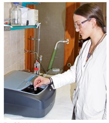
Figure 3: Sample insertion using a cell
